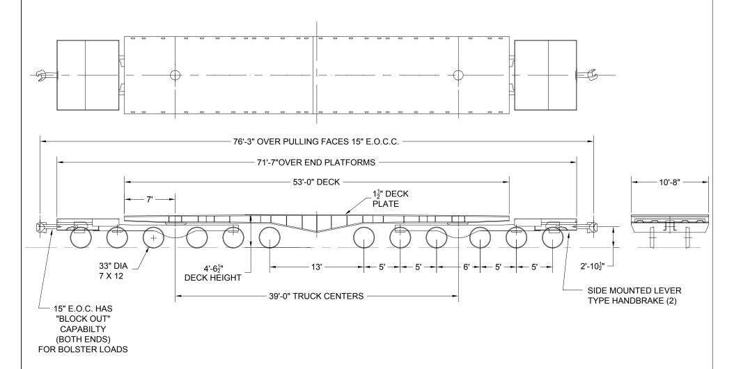
CAR WILL CARRY A CONCENTRATED LOAD AT THE CENTER OF THE CAR EQUAL TO THE LOAD LIMIT
