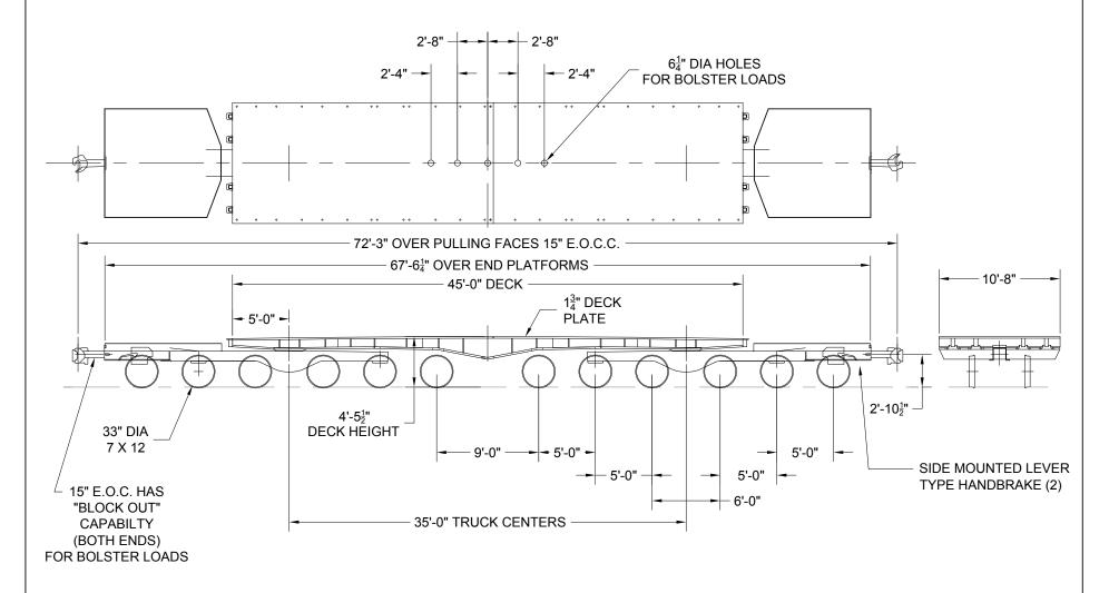
CAR WILL CARRY A CONCENTRATED LOAD AT THE CENTER OF THE CAR EQUAL TO THE LOAD LIMIT
