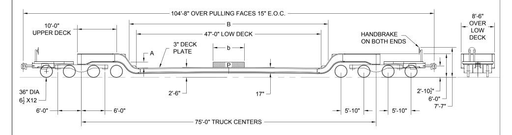
CAR WILL CARRY A CONCENTRATED LOAD AT THE CENTER OF THE CAR EQUAL TO THE LOAD LIMIT
